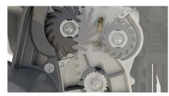
Feeder wheels grab the seed off the disk and place it onto the belt for delivery to the trench while maintaining superior singulation.
